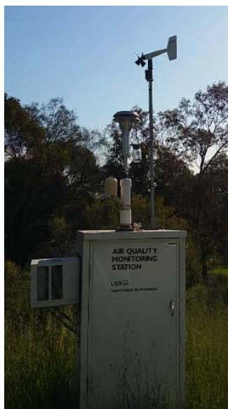
Air quality monitoring stations at the Angaston Quarry (left) and the Carrapateena Mine (right). (Photos 416717, 416716)
